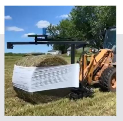
The Bale Buddy 2000 was designed to allow hay to be baled while there is up to 60% moisture in the hay. When the weather is uncooperative, this will save time waiting for the hay to dry and product with less hay spoilage.
